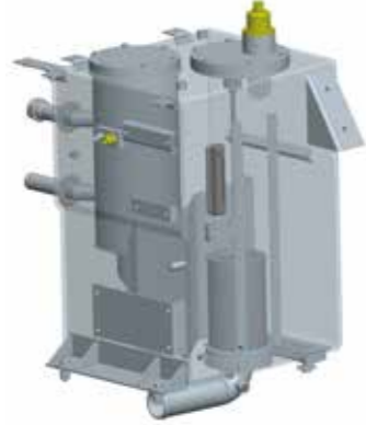
Fuel Tank with Additional Ribs and Pads
