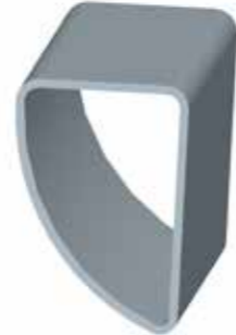
The Turntable Side Beam Adopts D-tube Structure
